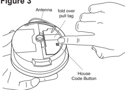
You can exit this mode by pressing the House Code button on one of the RF Alarms. Keep the button pressed until the blue light comes on solid and then release. Now re-affix the Alarm to its mounting plate.
