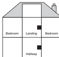
Position the Remote Control in a location that will allow it to be easily accessed. In the majority of installations this will be in a hallway, possibly next to the master bedroom.
