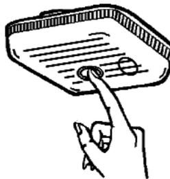
Press and hold the Test Button until the alarm sounds (it may take up to 10 seconds), (Figure 7). The alarm will stop sounding shortly after the button is released. If the alarm fails to sound, follow this checklist. Check the age of the unit - see “replace by” label on base of unit.
