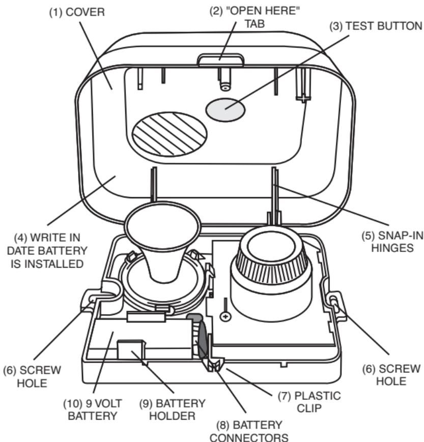
2. Place the Base on ceiling or wall exactly where you want to mount the unit. With a pencil, mark the location of the Screw Holes (6).
