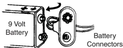
NOTE: You may hear a loud chirp when attaching the Battery Connectors to the Battery. N.B. The emergency light Smoke Alarm needs 2 batteries (see page 9 for details). Test the installed Smoke Alarm - see section 5(a) below.
