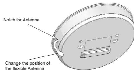
Figure 6 - Shows the Antenna moved to the outside of the Ei420 housing
