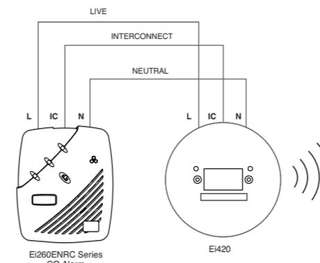
Figure 4a - The Ei420 used as an interface with an Ei261ENRC or an Ei261DENRC Carbon Monoxide Alarm
