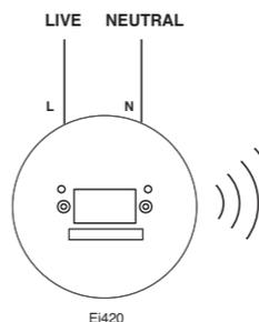
Figure 5 - The Ei420 used as a stand alone **RadioLINK** Repeater
